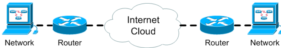
Figure 12.5. Router connections to the Internet cloud
